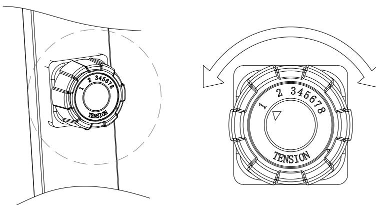
Turn the tension knob (17) clockwise to increase the resistance level, turn counterclockwise to decrease the resistance level. Level 1 is the lowest and level 8 is the highest
