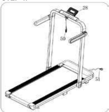
1. Put the Safety key (50) on the computer, and insert the Mobile phone holder (28) into the computer.
