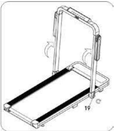
1. Loosen the Fixed pin (19) counterclockwise on both sides for 3-5 turns and push the upright upward in the direction shown on the left.
